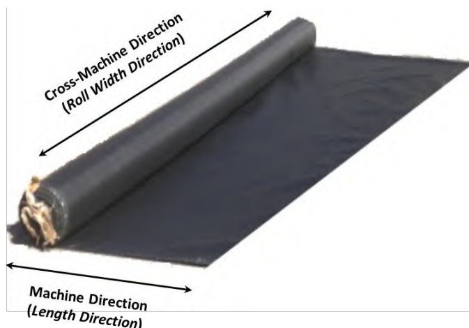
Figure 5. Illustration. Geosynthetic roll direction.
