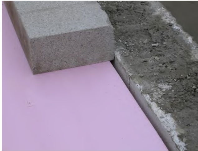
Figure 81. Photo. A 4-inch-thick concrete block on top of a foam board against the top of the CMU face block.
