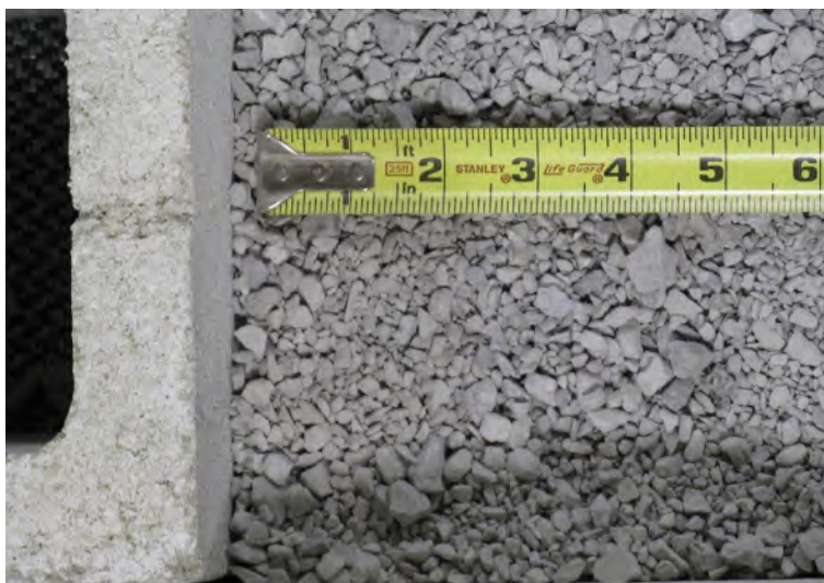
Figure 4. Photo. Sample open-graded aggregate.
